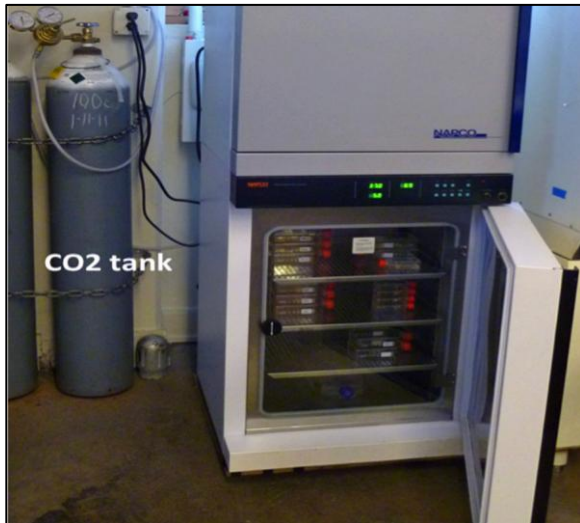
Figure 4- A cell culture incubator connected to the CO 2 tank.
