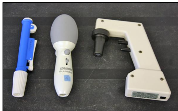
Figure 5- Manual (two on the left) and electrical (one on the right) pipette pumps.
